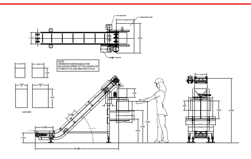
BULK FILL SYSTEM ENABLE TO FILL TOP LOAD RSC FOR A VARIETY OF APPLICATIONS. OPERATOR SHOWN TO ASSIST TOP/BOTTOM SEALING OF CASES IN A SEMI AUTOMATIC SYSTEM. WE WERE ABLE TO ELIMINATE MULTIPLE OPERATORS AND DECREASE GENERAL SAFETY CONCERNS.
