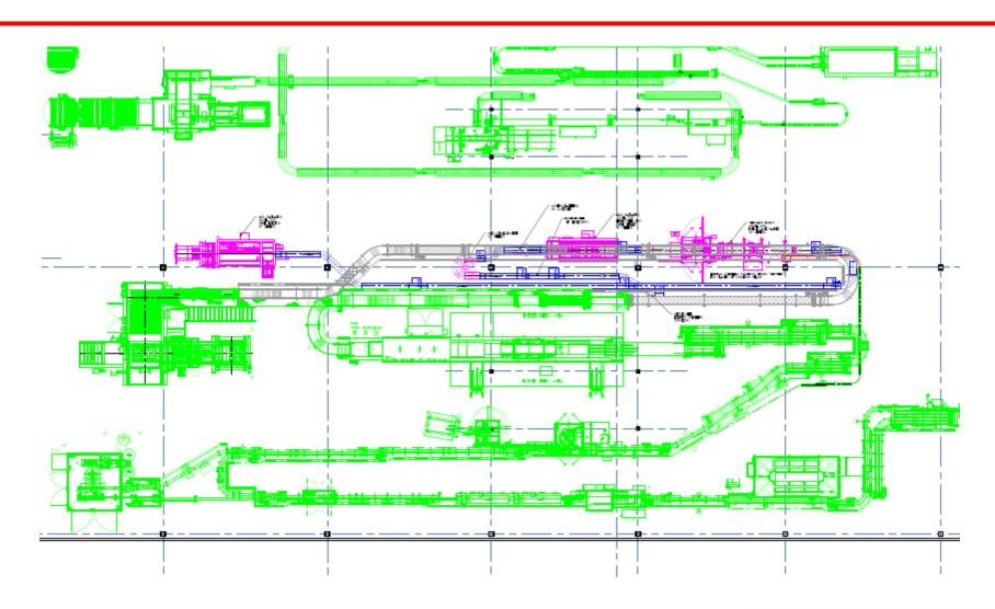
PRODUCT HANDLING SYSTEM TO ENABLE SPUR LINE TO BE ADDED INTO PRESENT LINE FOR MULTI PRODUCT HANDLING AND PACKAGING. CLUB PACKAGING REQUIREMENTS OF ASSORTED FLAVORS CAN BE PRE STAGED, COLLATED, AND PALLETIZED ACCORDINGLY.
